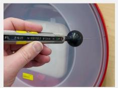
Image of the probe and picture of the probe used during the hazardous parts test.
