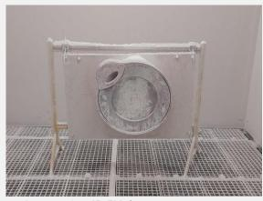
Image after IP 5X dust test
