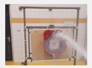
Image during IP X6 water test front
