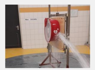
Image during IP X6 water test side
